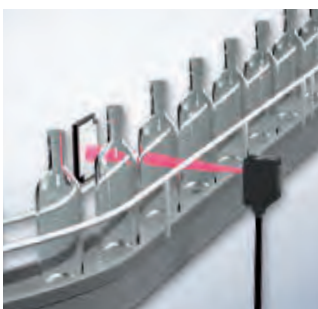
Easy adjustment for the detection of a large variety of transparent objects
