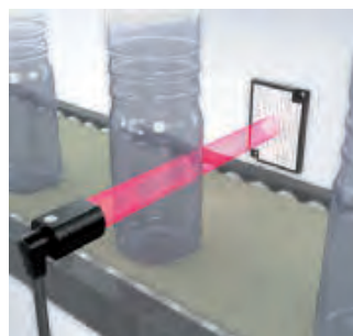
Reliable detection of PET bottles by unique p-opaquiring technology
