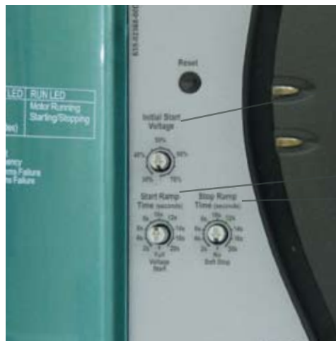
CSX control panel
