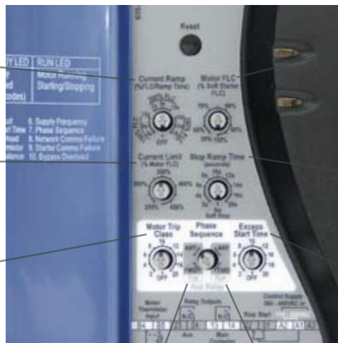
CSXi control panel
