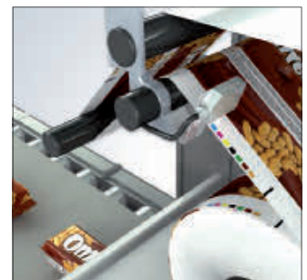
Reliable detection of standard or semi-transparent marks at normal or high speed
